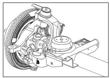
O The new bracket is designed to sit flush against the coil bucket. Make a cut inline with the front face of the coil bucket surface as shown.
