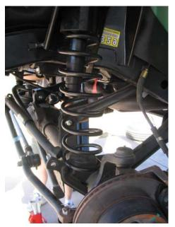
11. Now that the coil springs are installed go ahead and install your lifted front shocks( not supplied.) and raise up the axle and connect the sway bar end link and track bar to axle mount.
