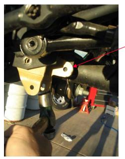
5. Using a drill, drill the 5/16 hole in the axle brake and install the bolt, washer and nut.using the stock bolt, install it in the stock location.(1)
