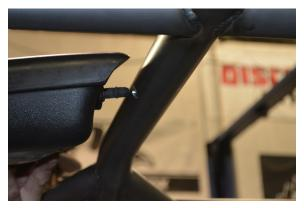
Make sure the two bolt holes are correctly marked on the Rear Down Bar, then remove the speaker pod, drill these holes to 7/32" and thread them with a 1/4-20 tap.
