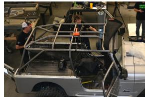
Check that each of the junctions where cage components meet are still correctly positioned, tubes line up with the correct etched markings or notches are correctly engaged into their slots on the adjoining pieces.
