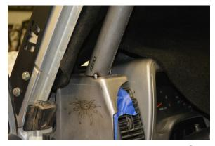
**29. (Optional) Install the Seatbelt Bar** <sup>(1)</sup> to the rearward side of the B-Pillars. Use the laser-etched assembly marks as guides to properly locate the tube junctions. If using custom seats and belts, you may adjust the height of the Seat Belt Bar (ignoring the laser etched assembly guides) to properly locate it for your specific setup. It may be necessary to temporarily set the seats back into place to determine the optimal height. Tack the Seatbelt Bar into place.
