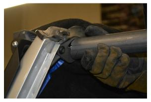
The other end of the Header Bar has lasercut slots that are designed to click into place on the tabs protruding from the end of the B-Pillar. Just set the Header Bar in place for now, do not tack or weld yet.
