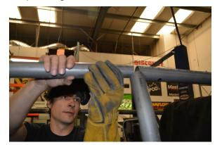
21. Install the B-Crossbar (2). Note that the B-Crossbar has two pairs of tab slots laser cut into the side of the tube, centered about half-way down its length. These tab slots will be oriented toward the FRONT of the Jeep when the B-Crossbar is set into place.
