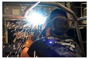
**34.** At some point it will be necessary to remove the cage from the Jeep in order to reach the last few areas that need to be welded.
