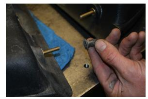
On the Poison Spyder cage there are drill locations already etched into the tubes for installing it. Pre-fit the speaker pods prior to drilling these holes. Check where the metal tang wants to poke through the B-Crossbar. IMPORTANT: There is already a laseretched mark for this hole, however we have found that there are some year models in
