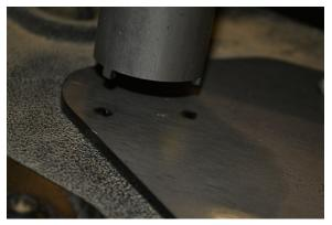
At the forward end of the Rear Down Bar, make sure that both it and the Header Bar seat properly into the notched end of the B-Pillar. There are tabs and slots cut into each piece to ensure proper fitment.
