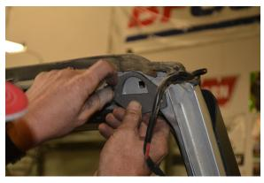
**10. Use the OE roll bar** hardware to Install the B-Pillar Mount Plate ② in the locations where the main hoop of the factory roll bar bolted in, just behind the door opening on either side.
