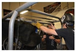
Note that the side of the Header Bar has been laser etched with a guide mark for proper placement of the A-Crossbar.
