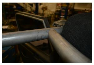
The slight bends at each end of the A-Crossbar should be oriented so that the center section of the Crossbar is bowed rearward, away from the windshield.
