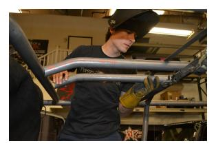
Note that the rearward end of each Forward Stringer has laser cut tabs that fit into slots in the side of the B-Crossbar. The forward end is located using laser-etched marks in the side of the A-Crossbar.
