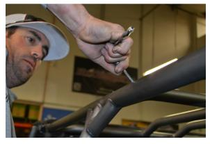
Re-install the speaker pod and use two (2) 1/4-20 X 3/4 Button Head Cap Screws with Flat Washers (hardware not included) to secure it to the Rear Down Bar.
