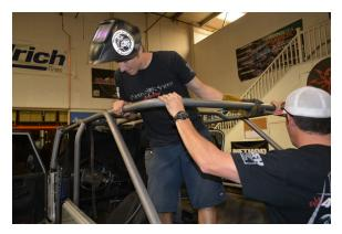
Once the C-Crossbar is correctly positioned, with a helper continuing to support the rearward side of the tube, tack it into place. The helper must continue to support the C-Crossbar through the following step.
