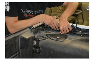
12. Install the Lower A-Pillars L&R ④. Bolt each Lower A-Pillar into place using the three Torx bolts you removed during Step 5 of the Factory Cage Removal process. Note that once installed, the Lower A-Pillars will NOT be oriented perpendicular to the Jeep. They will angle slightly inward. Be sure to test-fit the doors for proper closing, before proceeding.
