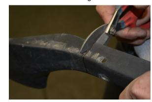
**38. If re-installing the upper door** surrounds for the OE soft top, there are drill marks already laser etched into the Header Bar tubes. Note that there are two center marks, which will vary depending on year model. Pre-fit your door surrounds to determine which marks are correct, then drill them out to install the door surrounds.
