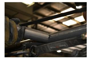
24. Once the Forward Stringers and A-Crossbar are positioned correctly, tack them together and to the Header Bars and B-Crossbar.
