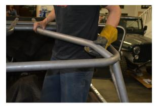
There are alignment marks etched into each of these tubes to properly locate and align them.
