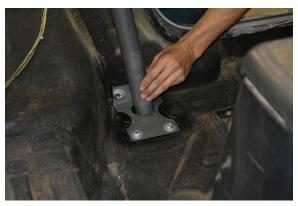
**15. Insert a B-Pillar Bolt Sleeve** (2) into the B-Pillar, through the hole provided that aligns with the sheet metal roll bar bracket that is attached to the tub. It may be necessary to sand or de-bur the ends of the sleeve and/ or the edges of the laser cut holes in the B-Pillar. Use a soft dead-blow mallet to tap
