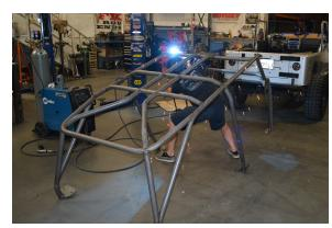
**35. Install the 90° Gussets** (2) at the junction of the B-Pillar, B-Crossbar, Header Bar and Rear Down Bar.
