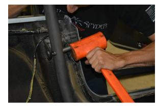
**16. Insert a 1/2-13 X 3-3/4** Gr8 Hex Head Cap Screw through a 1/2" Flat Washer, through the hole in the sheet metal roll bar bracket, through another 1/2" Flat Washer, then through the B-Pillar Bolt Sleeve. Install a 1/2-13 Gr8 Nylon Insert Lock Nut on to the bolt where it protrudes through the sleeve, leaving it only finger-tight for now.
