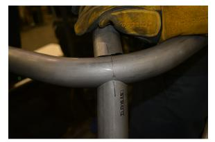
Once the Rear Stingers are correctly positioned, tack them in place to the B-Crossbar and C-Crossbar.
