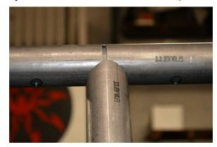
At the other end of the Rear Down Bar, insert the tabs that were laser cut into the end of the tube, into the corresponding slots cut into the C-Pillar Mount Plate that was installed
