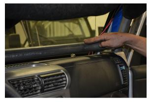
With all three pieces (both Upper A-Pillar Tubes and the Dash Bar) positioned, tack them into place.
