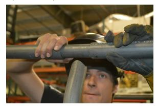
Take care to make sure the sleeve inserts into the Header Bar so that its edge is past the rosette hole in the bottom of the Header Bar, while the other end is still past the rosette hole in the Rear Down Bar. Slide the Header Bar and the Rear Down Bar together until they meet (the will be slightly separated by tabs cut into the ends of the tubes).
