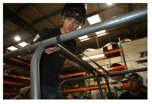
**22. Set the A-Crossbar** (1) in place, spanning between the two Header Bars, toward the front, near the windshield.
