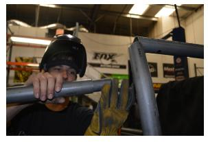
Insert the other end of the Header Bar Sleeve into the Header Bar that was set into place in a previous step.
