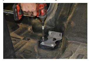
**11. Install the C-Pillar Mount Plates** ③ where the factory roll bar bolted in at the rear corners. Orient the plates with the rounded point edge facing the rear of the Jeep. Secure them using the OE hardware, leave the bolts slightly loose.
