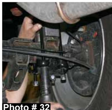
37. **Rear Leaf Spring Installation:** Remove the OEM leaf springs & install the new Skyjacker leaf springs on top of the OEM rear blocks with the thicker portion of the degree shim facing towards the rear of the vehicle. **Note:** It will be necessary to lower the gas tank to gain access to the OEM forward leaf spring mounting bolt.
