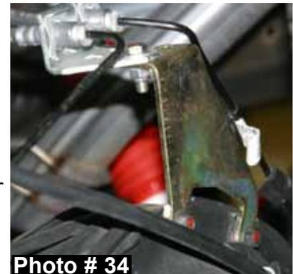
40. Remove the OEM emergency cable bracket from the driver side frame & install the new Skyjacker emergency cable bracket to the frame using the OEM hardware. Attach the OEM emergency cable to the new emergency cable bracket using the supplied 5/16" x 1" fine thread bolt, SAE washer, USS washer, & nut. (See Photo # 35)
