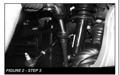
4. Disconnect the tie rod from the factory knuckle. Save hardware. SEE FIGURE 3
