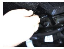
Reinstall the inner fender well using the stock hardware where applicable.
