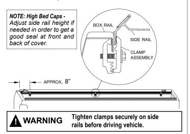
STEP 2: For optimum latching performance and cover fit, side rails must be level. To adjust rails, loosen screws and reposition male clamps higher or lower. Tighten all clamps.
