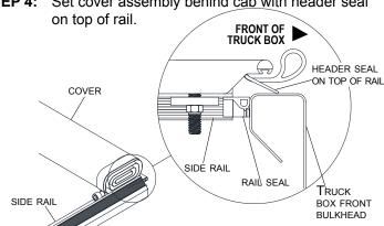
STEP 5: Tighten bolts but do not over tighten. Header must be free to slide.
