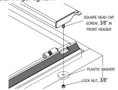
**STEP 4:** Set cover assembly behind cab with header seal
