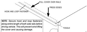
STEP 8: To release cover, Trigger pull rear release toggle. Start rolling cover toward cab making sure both sides of cover roll evenly. For best results leave unrolled portion of cover attached to the hook and loop fasteners while
