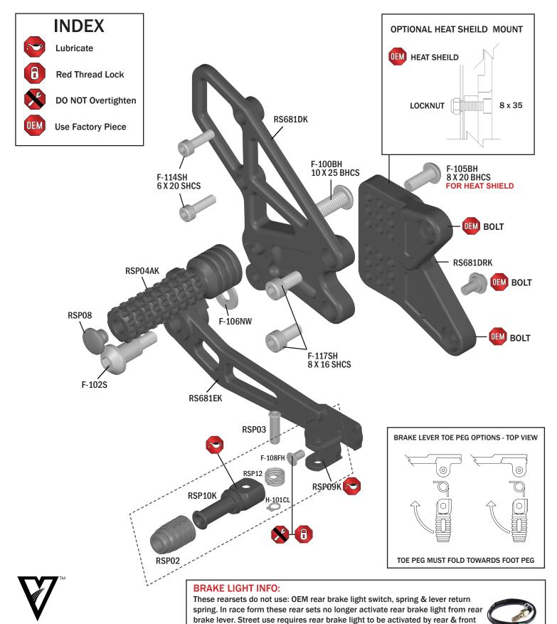
brake levers. To achieve rear brake light activation from rear brake lever use
