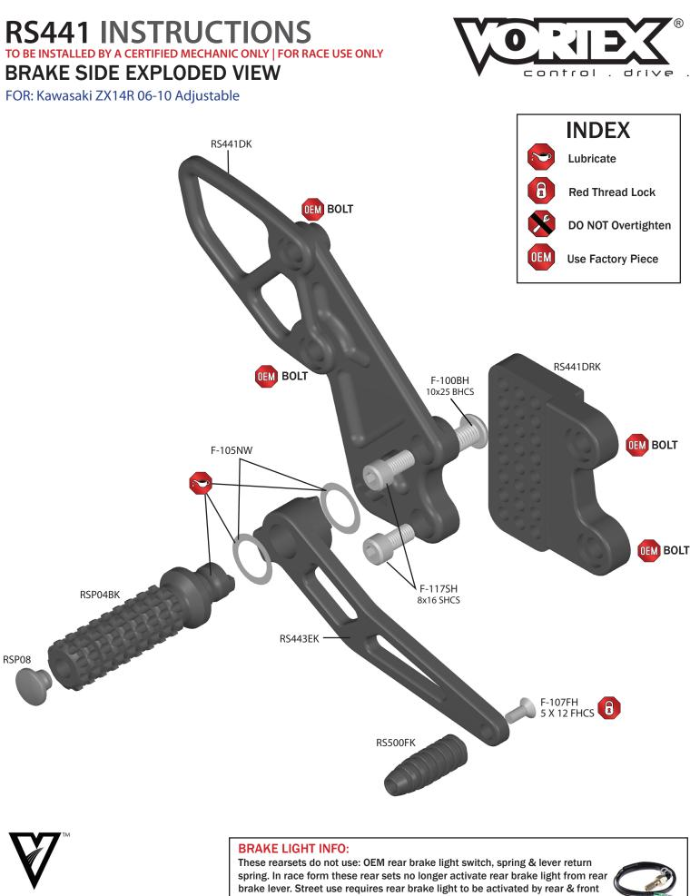
1.800.440.3559 www.VORTEXRACING.com brake levers. To achieve rear brake light activation from rear brake lever use Vortex in-line pressure switch RS100.
