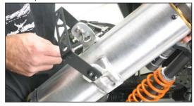
Install TBR muffler assembly to the UTV frame using OEM bolts and nuts.
