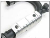
4. Using the two OEM bolts and washers, install a lock washer as shown and install OEM heat shield on TBR mid-pipe. Re-install bumper stop.
