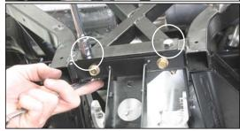
8. Install barrel clamp on end of slip-tube. Install mid-pipe.
