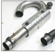
Attach slip-tube to TBR muffler using the two-piece X-ring and four 6x20mm socket head cap screws and split lock washers provided.
