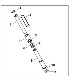
for 1936–2014 Harley-Davidson<sup>®</sup> & S&S Engines Refer to the diagram to determine the correct **10.** Lower pushrod seal. a. Harley-Davidson<sup>®</sup> knucklehead and S&S positions for pushrod cover components, and the correct type of seals for various engine styles. Note that depending on the kit you have purchased, not all the components may be b. Harley Davidson® panhead, shovel, and included. In these cases it is expected that stock components will be reused. In addition, not all
