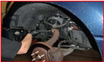
Strike the upper ball joint boss with a dead blow hammer to dislodge the taper. Remove the upper ball join nut hardware and separate the upper control arm from the knuckle. Loosen but do not remove the upper control arm hardware.
