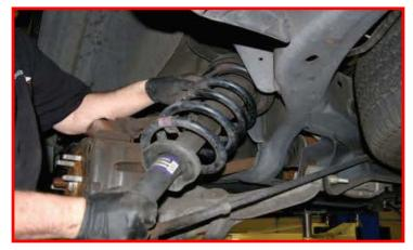
Install the ReadyLIFT strut extension to the strut using the provided M10 flange nuts. Torque to 30 ft-lbs.
