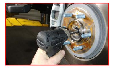
Locate the vacuum line at the hub actuator and remove.
