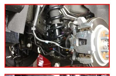
Remove the plastic clips from the control arm and frame rail. Let the ABS harness hang out of the way. Place a suitable jack under the lower strut mount.
