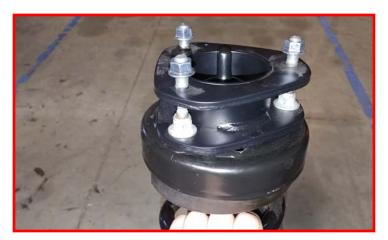
Install the completed strut assembly to the frame using the provided M10 -1.25 Flange nuts. Do not tighten at this time.
