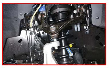
Install the vacuum line to the vacuum actuator by pressing into place.
