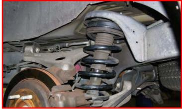
Loosen but do not remove the upper and lower control arm hardware at the frame and knuckle. Remove the tie rod end from the knuckle. Strike the tie rod boss with a dead blow hammer to dislodge the taper. Separate the tie rod from the knuckle.
