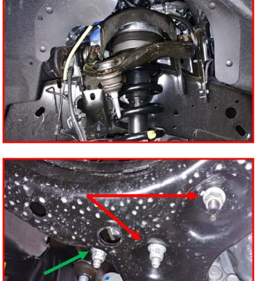
Raise the lower control arm up while guiding the lower strut into place. Install using the factory hardware. Install the sway bar end link using the factory hardware. Torque all to 45 ft-lbs.
