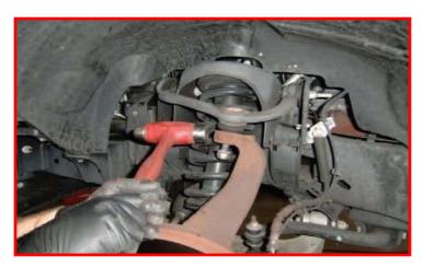
Install the strut to the frame using the provided M10 flange nuts. Do not tighten at this time.
