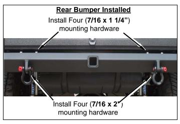
2. Align and Center bumper assembly(Be sure that rear hatch clears bumper), tighten all six mounting bolts.
