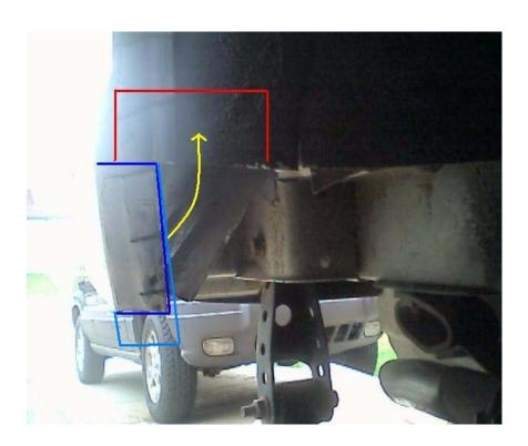
Step 6: The photo below represents the inner piece being folded up and preparing to fold up the outer section:
