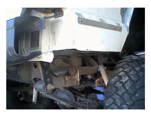
Step 3: Next Step is to cut where that darker line was shown in the first picture; which will result in the photo below: (Note: You will need to cut through the inner part of the fender as well.)
