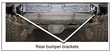
**b.** Place two *kit* spacers (1/2") on to *kit* bumper mounting bracket.
