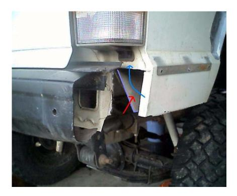
Step 5: The photo below represents the inner part of the fender after being cut. The darker outlined piece is the section that will fold up and relocate where the lighter outlined box is shown:
