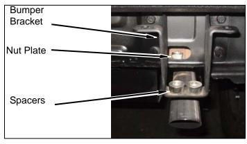
c. Install kit nut plate(Two 1/2" nuts weld on a plate) into frame rail through access hole in frame. Using supplied kit hardware, two 1/2" bolts & washers, to install anchore strap on driver's & passenger's side frame mounts.
