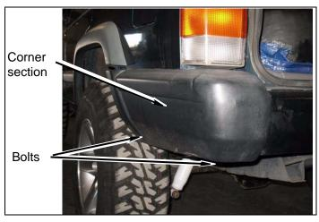
**c. 84-01:** Remove eight bolts from center section bumper brackets (right & left) at frame and remove bumper.
