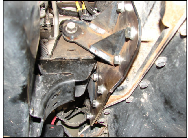
PS Block Bracket Installed
