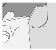
IMPORTANT: It should not be necessary to grind all the way through the steel bracket. Only remove enough material to eliminate the interference problem.
