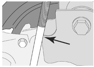
If interference between the control arm bracket and Connecting Rod (A) is discovered, it will be necessary to clearance the bracket per the following instructions.
