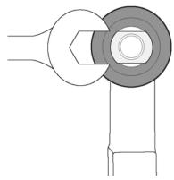
On the upper Rod Ends (B) only, cut the excess thread material from the mounting stud so that none of the threaded portion protrudes beyond Flanged Locking Nut (D).
