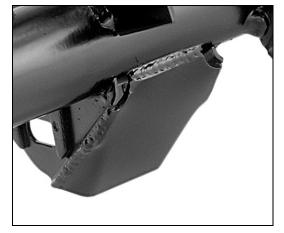
O Once all welding is complete, spray paint any bare metal on MiniSkids, suspension arm brackets, and axle tube to prevent corrosion. All exposed metal must be <u>completely</u> covered.
