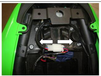
2. Unplug turn signals, and remove the side tail fairings.
