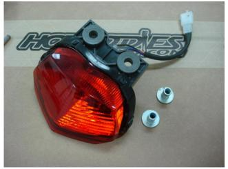
5. Remove metal sleeves from the rubber grommets on the taillight.
