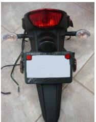
4. Remove the mud flap from the bike, and unbolt the taillight from mud flap.
