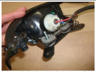
7. Connect the bracket and stock trim piece to the taillight as shown.
