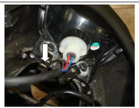
3. Unbolt the mud flap from sub frame and unplug the taillight from the bike.
