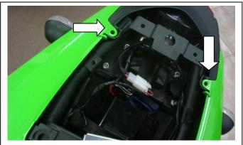
1. Remove the rear seat, and bolts securing the tail fairing.
