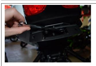
8) 2 of the 10mm mounting bolts will need to mounting from the inside of the tag bracket as shown. DO NOT OVERTIGHTEN USE THREADLOCK!
