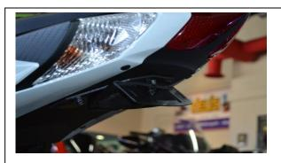
10) Re-install right side tail fairing using the 4 stock pop rivets 1 phillips screw. Re-install the rider and passenger seats as well as the covers to access the seat bolts and then attach your license plate and you're done!
