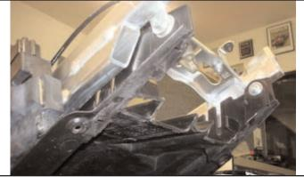
**4)** Re-attach glovebox, replace all bodywork with fasteners loosely installed. Install undertail left side first, then right side, be careful not to scratch, or crack undertail. Use plastic screw rivets to hold undertail in place. Insert lock into undertail using stock lock mounting clip, make sure the lock is in the correct position with the lock cable arm to function properly.
