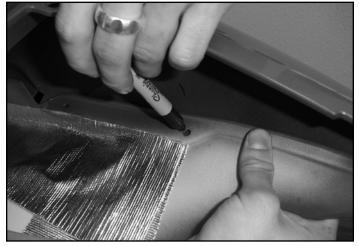
2) When tail section body work is removed, line up the undertail with tail section carefully marking holes from bottom to top, respectively on each side. Make sure tail is correctly lined up with tail section.
