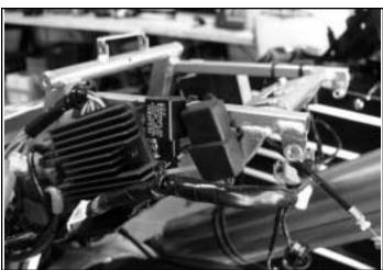
4) Attach the loose relays to the sides of the subframe using 2 zip ties.
