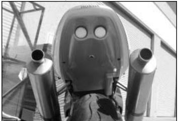
6) Inset lock into undertail using stock lock mounting clip, make sure the lock is in the correct position with the lock cable arm to function properly. Insert undertail left side first, then right side, be carefull not to crack or scratch undertail. Use your stock plastic screw rivets to hold undertail in place. Attach lock cable to lock, check movement, adjust if necessary. Tighten all hardware on tail section, attach seat.
