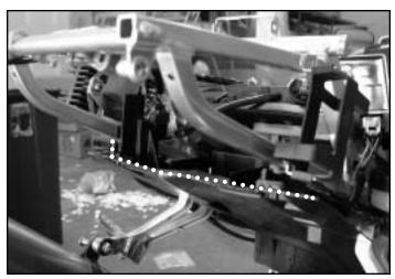
2) Using a "Dremel" tool or cutting disc (this can also be done using a sharp edged knife, but is not recommended), remove the plastic shown in the photos to the above and below. Your subframe may be different but the cutting position is the same on all years. Be sure to take your time cutting, so that you don't cut away any more plastic than necessary.
