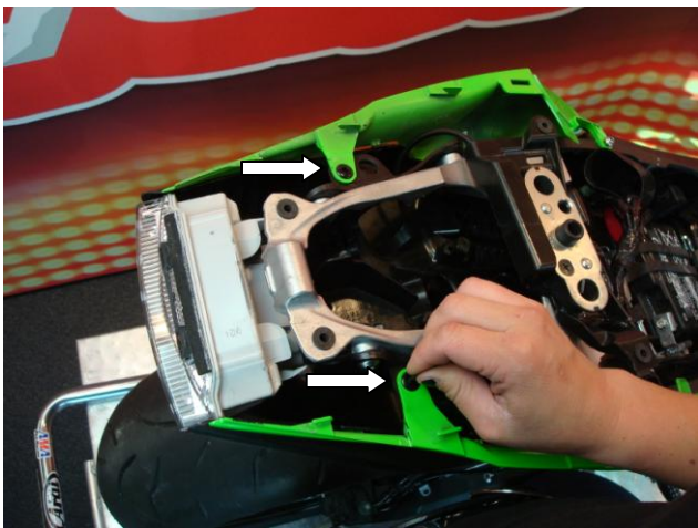
7. Remove the back 2 pop rivets.
