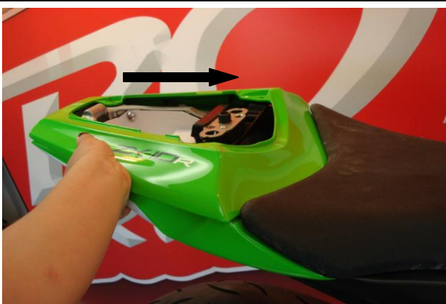
33. Install the top tail fairing. Squeeze both sides as you slide into place. Ensure all tabs are engaged
