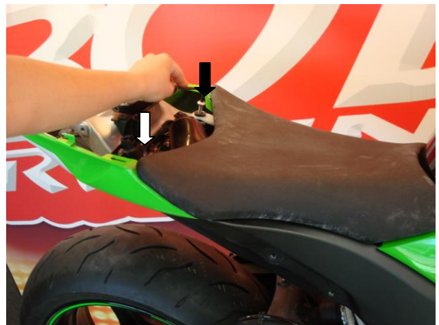
32. Install the front seat, using the stock hardware.
