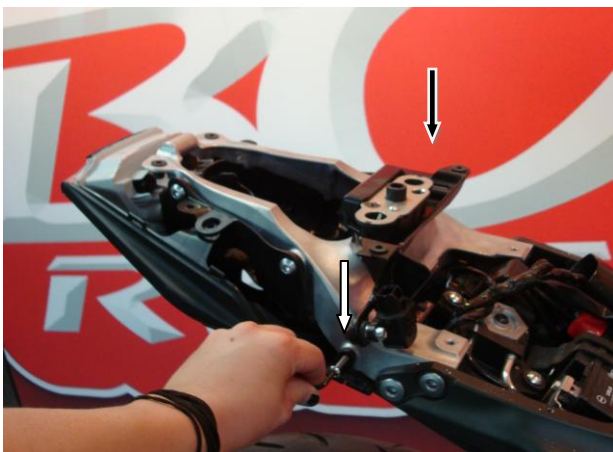
9. Remove fairings, and back bolts from stock undertail.
