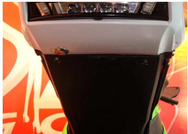
26. Install the undertail, making sure the tabs are inside the battery tray.
