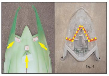
8) Peel off adhesive cover, and attach tail light to the new undertail.\*For smoke undertail using clear double sided tape that is provided apply to your tail light (as seen in Fig. 4) and then place on new smoke undertail. Place new undertail over tip of subframe and mount rear bolt loosely and install stock pop rivets at the bottom of the new undertail. Re-connect tail light and wire in new signals and license plate light. \*For permanant assmbly apply black or clear silicone around light.\*
