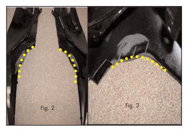
5) Trim inner tabs of tail section as seen in Fig. 2. Closer view in Fig. 3.
