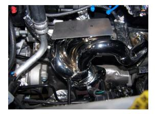
5. NOW ON PASSENGER SIDE REMOVE STOCK SHIELDS, SPARK PLUG WIRES, AND MANIFOLD. MAKE SURE TO CLEAN HEAD SURFACE OF ANY DEBRIS.
