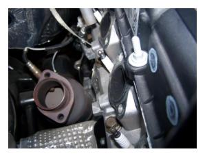
6. NOW INSTALL GIBSON HEADER WITH SUPPLIED GASKET RE-USING STOCK BOLTS TORQUING TO 30-35 FT-LBS FROM CENTER OUT. AFTER HEADER IS IN PLACE, USE SUPPLIED HEAT WRAP ON SPARK PLUG WIRES AND ZIP TIE TO KEEP AWAY FROM HEADER FOR HEAT PROTECTION. (NOTE: MAKE SURE ALL WIRES AND HOSES HAVE PROPER CLEARANCE FROM HEADER!)
