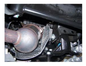
2. NOW STARTING UP TOP ON THE DRIVER SIDE, REMOVE STEERING SHAFT FOR REMOVAL OF FACTORY MANIFOLDS AND INSTALLATION OF HEADER. DISCONNECT ALL SPARK PLUG WIRES, REMOVE FACTORY HEAT SHIELDS AND MANIFOLD. MAKE SURE CYLINDER HEAD SURFACE IS CLEAN OF ANY DEBRIS BEFORE INSTALLATION OF HEADER.
