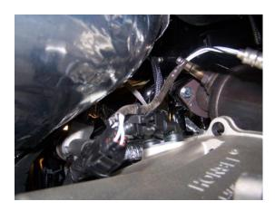
8. PERIODICALLY CHECK AND RETIGHTEN THE HEADER BOLTS.
