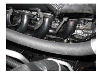
10) WRAP SPARK PLUG BOOT WITH HEAT WRAP PROVIDED AND RE-INSTALL. USING THE NUTS AND BOLTS PROVIDED, RECONNECT THE HEADERS TO THE STOCK EXHAUST UNDERNEATH THE VEHICLE.
