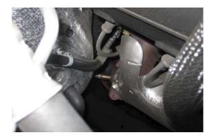
8) REMOVE THE FIVE BOLTS ATTACHING THE MANIFOLD TO THE HEAD. REMOVE THE MANIFOLD FROM THE TOP OF THE VEHICLE.CLEAN THE SURFACE OF THE HEAD. REMOVE ANY CARBON DEPOSITS THAT MAY BE ON THE HEAD.PREPARE THE SUPPLIED HEADER BOLTS WITH ANTI-SEIZE TO THE THREADS.
