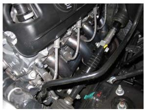
6) RE-INSTALL THE SPARK PLUG WIRES, DIP STICK TUBE, AND RECONNECT THE STEERING SHAFT ON THE ALIGNMENT MARK.
