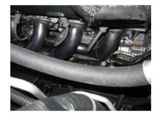
10) WRAP SPARK PLUG BOOT WITH HEAT WRAP PROVIDED AND RE-INSTALL. USING THE NUTS AND BOLTS PROVIDED, RECONNECT THE HEADERS TO THE STOCK EXHAUST UNDERNEATH THE VEHICLE.
