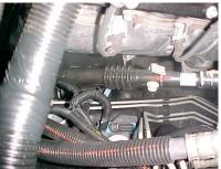
3. On the topside of driver side and passenger side: Disconnect the spark plug wires by grasping and gently twisting the spark plug wire boots. Do not pull on the wires. Set the wires and looms up out of the way. Brush or blow away any debris that may have collected around the manifolds and spark plugs. This will help prevent foreign matter from entering the combustion chambers when the manifolds are removed. Removal of the spark plugs is necessary to avoid accidental spark plug breakage.
