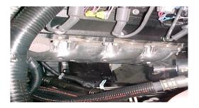
5. Now Repeat #'s 3-4 on passenger side. (Note: The EGR hose is at rear of manifold). You should remove air cleaner assembly so you have room to work, unbolt dipstick tube and gently pull upward.
