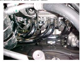
10) RE-INSTALL THE DIPSTICK TUBE. WRAP SPARK PLUG BOOT WITH HEAT WRAP PROVIDED AND RE-INSTALL. USING THE NUTS AND BOLTS PROVIDED, RECONNECT THE HEADERS TO THE STOCK EXHAUST UNDERNEATH THE VEHICLE.
