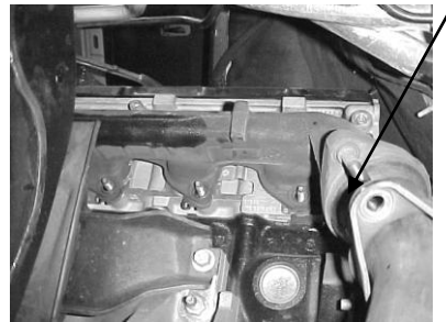
#6. FACTORY FLANGE CONNECTION. DISCONNECTING POINT.
