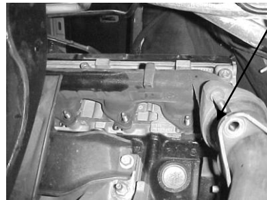
#6. FACTORY FLANGE CONNECTION. DISCONNECTING POINT.
