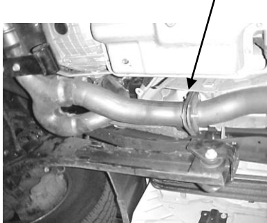
#1. FACTORY Y-PIPE 3-BOLT FLANGE.
