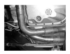
On suburbans there is an extra set of coolant lines passing by the headers on the passenger side. Take care to keep these back away from the headers so there is no contact with the tubes.
