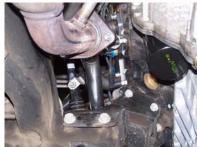
**IT IS CRITICAL** that all bolts be re-tightened HOT after about 20 minutes of operation to prevent gasket failure.
