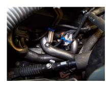
6. Using the supplied fasteners, bolt the Header to the bottom flange but do not tighten at this time. The nuts are jam nuts. Therefore they will not spin freely. This is normal. Torque headers to 30-35 ft/lbs after both headers are installed.
