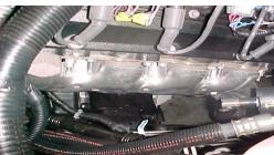
4. Remove all fasteners and studs from head. Remove manifold from top and install header and hardware through top of engine compartment. Also prepare header bolts with anti-seize to the threads.
