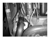
6. Remove O2 sensors cut head pipes. Driver side, cut 11 ½" forward from weld on front side of converter. Passenger side cut 19 ¾" forward of flange. Use hacksaw or power saw, 18 tooth blade is best, (use eye protection) file inside so no burs will interfere with new head pipe.
