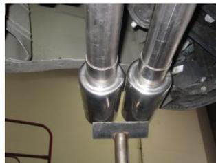
7. Install your black ceramic coated tips. Proceed to the next sheet on how to install your deegan 38 badges. After you have checked for clearances go back and tighten all nuts, bolts and clamps.
