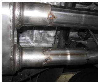
4. Install muffler #B onto headpipe #A 1.5-2". Use a jack stand to support the muffler. Use clamp #f to secure muffler to headpipe. Do not tighten.
