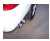
**7.** Attach both tailpipes using bolt kit #H. Position driver side tailpipe on top of passenger side.
