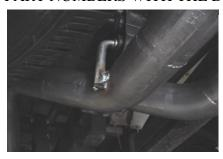
SLIDE DRIVERS SIDE TAILPIPE #D INTO MUFFLER 1-1/2" TO 2". INSERT WELDED HANGER INTO RUBBER GROMMET.
