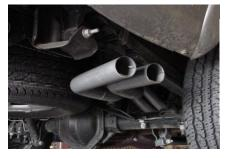
USE BOLT KIT #J TO SECURE TAILPIPES TOGETHER. THE PASSENGER SIDE TAILPIPE WILL BE ON THE BOTTOM.
