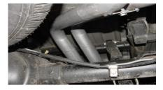
SLIDE PASSENGER SIDE TAILPIPE #E INTO MUFFLER 1-1/2" TO 2". USE CLAMP #I TO SECURE TAILPIPE TO MUFFLER. DO NOT TIGHTEN.
