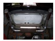
**7.** Next, install the exit pipes #C. Use clamp #E to secure tail pipes.
