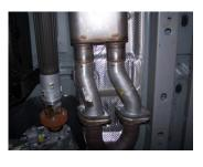
3. Install passenger side headpipe #A onto stock flanges using bolt kit #H. Do not tighten. Then install driver side headpipe #B using bolt kit #H. Do not tighten.
