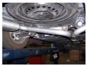
6. Next, install the driver side muffler assembly #B onto the Y-pipe. Insert welded hangers into rubber grommets. Use clamp #D to secure. Do not tighten.
