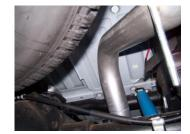
6. Slide the over axle tailpipe #C into the muffler 1.5-2". Use clamp #E to secure tailpipe to muffler. Do not tighten. Insert welded hangers into rubber grommets.
