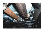
3. Install headpipe #A onto your existing stock front headpipe using stock hardware to secure pipes together. Do not tighten. Insert welded hangers into rubber grommets.
