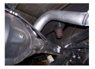
muffler. Use clamp #E to secure the muffler to the headpipe. Do not tighten. Muffler inlet is looking into the louvers.
