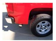
8. Install stainless steel tip. Clamp down. When you have everything in place, firmly tighten all bolts and clamps down securely. Use stainless steel or aluminum cleaner to polish tips. Inspect all fasteners after 25-50 miles of operation and re-tighten as necessary.
