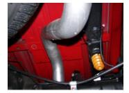
5. Install the over axle tailpipe #C onto the outlet of the muffler 1.5"-2" using clamp #E to secure pipe to muffler. Insert welded hanger into rubber grommet.
