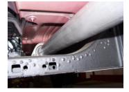
3. Bolt adapter pipe #G to the stock flange re-using the factory clamp. Insert welded hanger into rubber grommet. Do not tighten, just make snug.
