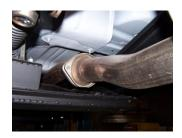
2. To remove stock exhaust unbolt it from the 2 bolt flange located in front of your stock muffler. You will reuse the factory nuts. Cut your stock tailpipe off for easier removal of stock exhaust. Use WD-40 to disengage hangers from rubber grommets. Do not damage or remove the rubber grommets as you will reuse them to mount your new system.
