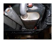
**4.** Install muffler onto head pipe #A. 11/2"-2" with the louvers facing towards the converter. Use a jack stand to support the muffler. Use clamp #E to secure the muffler to the headpipe. DO NOT TIGHTEN. Muffler inlet is looking into the louvers. Outlet will be on the drivers side.
