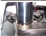
**2.** To install driver side muffler assembly #A, insert welded hangers into rubber grommets. Use clamp #C to secure to stock tailpipe. Adjust muffler assembly to best suit your vehicle and tighten clamp.
