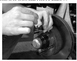
12. Place the tie rod end into the spindle. Reinstall the castle nut and torque it to 35 ft/lbs. Aligning it with one of the cotter pin holes in the tie rod end. Install one of the new supplied cotter pins. SEE PHOTOS BELOW.
