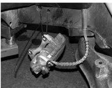
3. Support the lower control arm (LCA) with a floor jack, using enough tension to compress the control arm ¼". Remove the cotter pin and castle nut from the tie rod end at the spindle. Separate the tie rod end from the spindle using a tie rod puller. Remove the dust cap from the rotor using a hammer and a chisel. DO NOT DAMAGE THE CAP, YOU WILL BE REINSTALLING IT LATER. Slide the rotor and bearings off the spindle, keep the bearings in the spindle. SEE PHOTO BELOW AND IN NEXT COLUMN.
