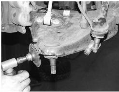
7. On models with front ABS, attach the sensor to the spindle in the provided hole. Use a ¼" x 1 ¾" bolt, ¼" lock washer and ¼" flat washer to mount the sensor. There are 2
