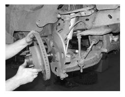
4. If this truck is equipped with front ABS, separate the line from the spindle and set the sensor aside. Remove the top clinch bolt from the spindle. Remove the cotter pin and castle nut from the lower ball joint. Separate the lower ball joint from the spindle and slide the spindle off the ball joints. SEE PHOTOS BELOW.
