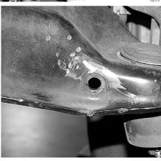
6. Using a die grinder with a cutoff wheel, remove approximately ¼" from the front lip of the lower control arm. Remove any burrs using a sander. SEE PHOTOS BELOW.
